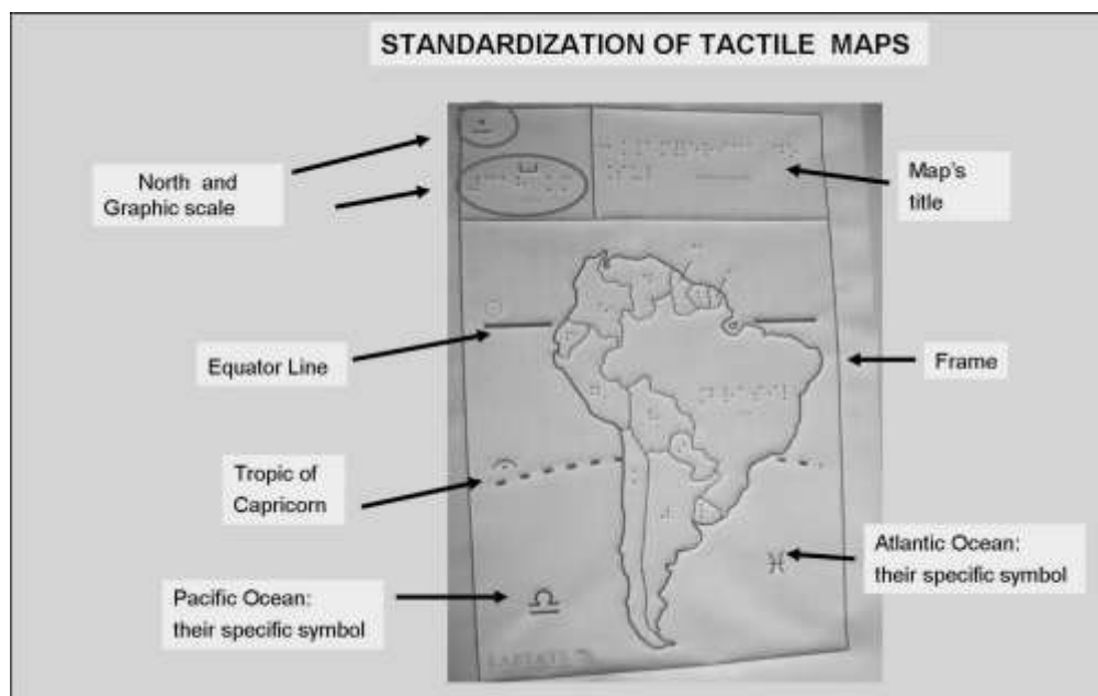
Figure 10: Standard layout for the small scale maps produced in microcapsule acetate paper and the example applied to South America in microcapsule paper, whose original size is that of a A4 paper format
